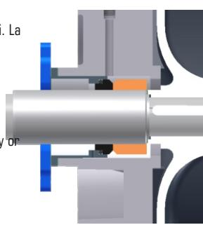
**EN** Single seal for dirty or viscous liquids. its position, close to the impeller, facilitates lubrication.
